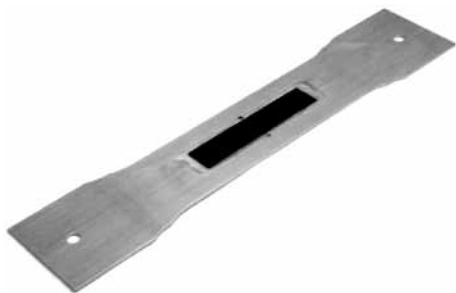
Figure 1. Test specimen with artificial cut cover by composite patch
