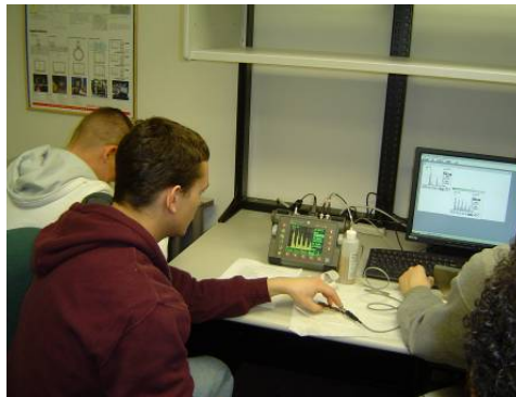
Figure 4. Calibration of the flaw detectors using a straight-beam probe.
