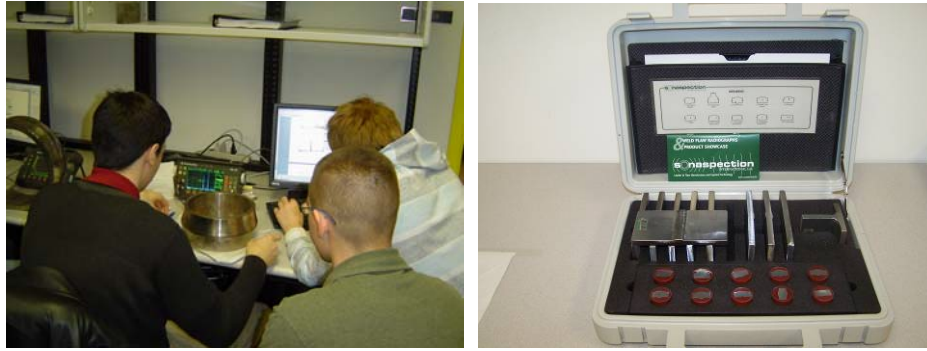
Figure 2. Large diameter (320 mm) bearing (left) and welding samples (right).
