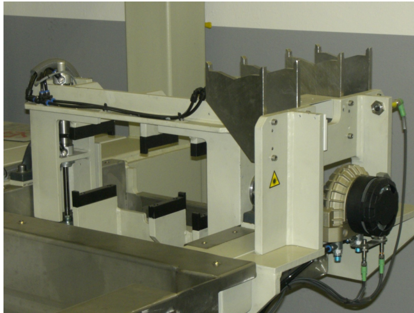
Figure Turning device. Thick specimens must be tested from two sides and are therefore turned (outside the tank).
