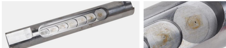
Figure Test Blocks. Round bar of diameter 60 mm and with seven 1 mm flat bottom holes in different depths.
