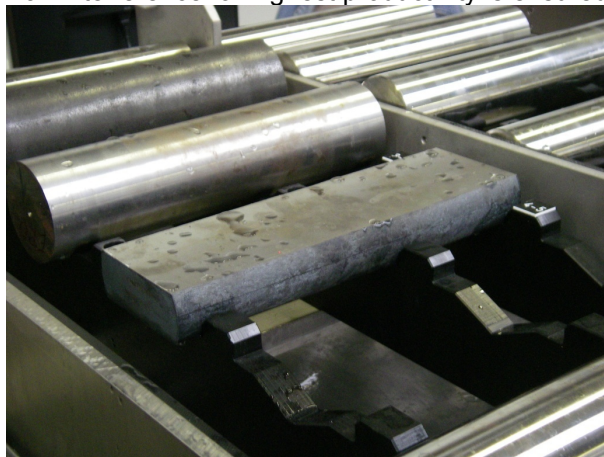
Figure Specimen Carriage. Up to 20 specimens of varying shape can be placed into the carriages and are sequentially tested one by one.
