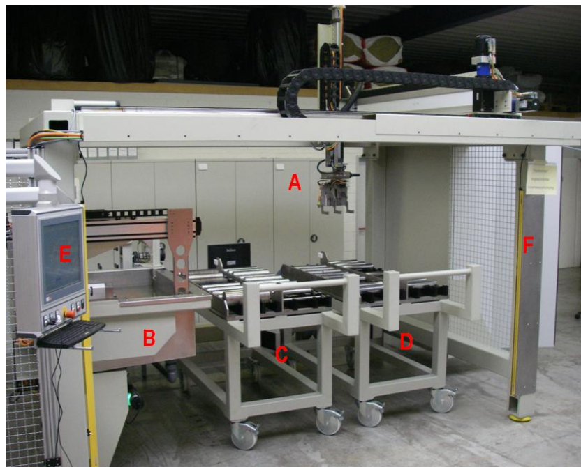
Figure Test Portal. Fully automated system for steel cleanliness inspection. A = gripper for specimen loading and discharging, B = immersion test tank, C = specimen carriage no1, D = specimen carriage no2, E = monitor for electrical and ultrasonic control, and F = safety curtain.
