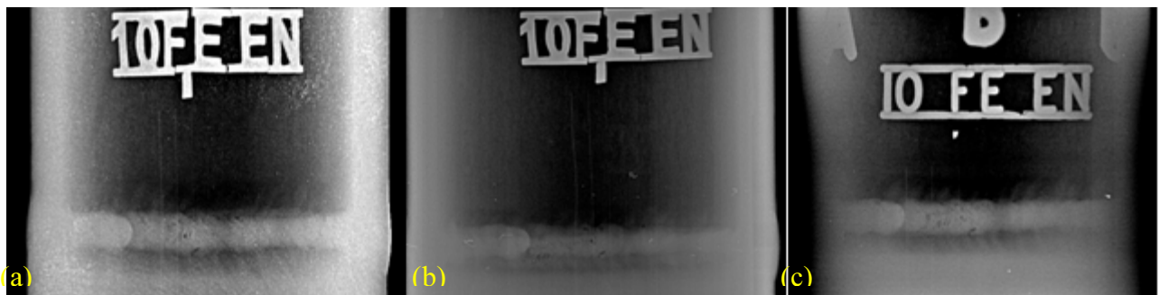
Figure 6 – Spool Ø2½" sch80, joint 03 position B : (a) Kodak System; (b)Dürr System; (c) GEIT System. High Pass Filter
