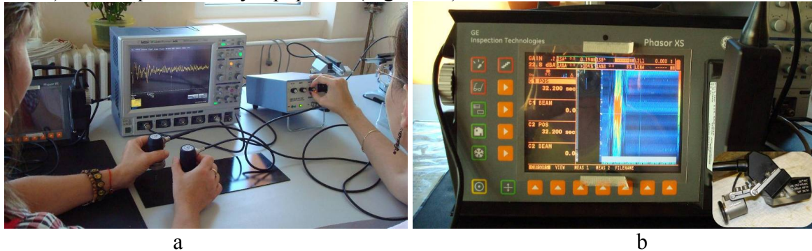
Figure 7. The experimental set-up: a) Equipment with Lamb wave generated by Hertzian contact; b) Phasor XS
