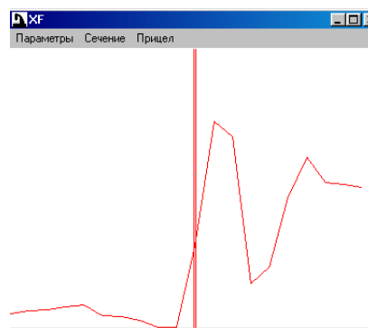
Fig. 2 Light intensity distribution of Fresnel diffraction pattern by real object's edge
