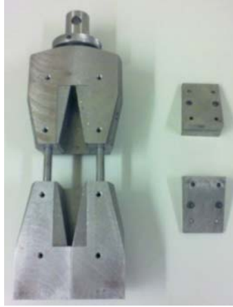
Fig. 1 – Compression-after impact (CAI) test fixture.
