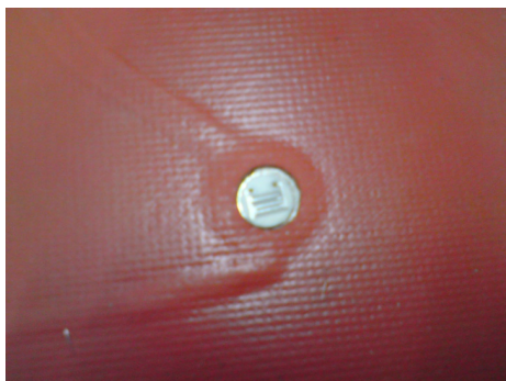
Figure 13 a: Dielectric sensor embedded into a blanket. The coupling thermocouple can be vaguely observed.
