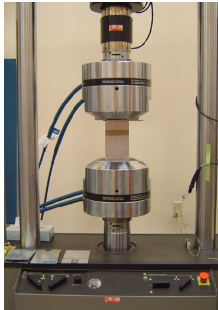
Figure 5: Weak Bond Specimen Mounted in Uniaxial Mechanical Test Machine to Determine Bond Strength
