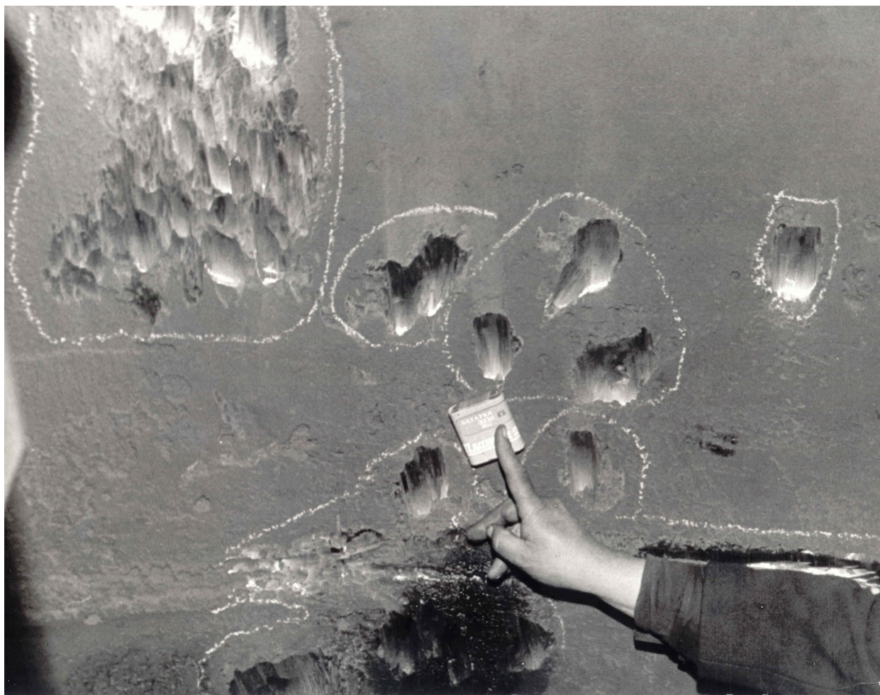
Fig. 7. Corrosion defeat of monoethanolamine clearing regenerator.
