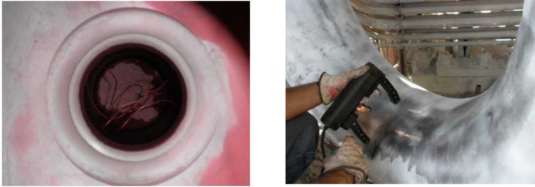
Figure 2: PT and MT being performed on a Steam Turbine unit.
