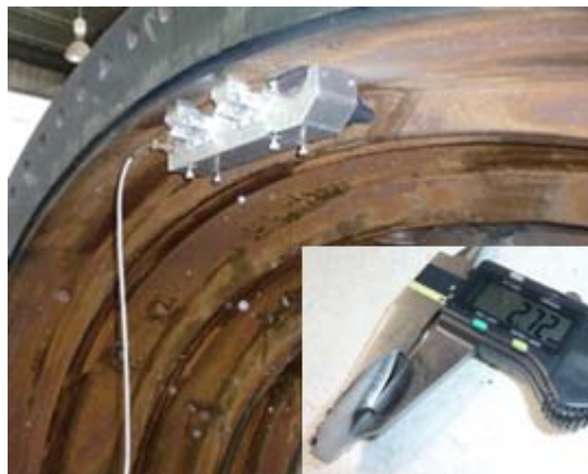
Figure 7: Siemens scoop (boat) sample tool removing a sample from a gas turbine cylinder.
