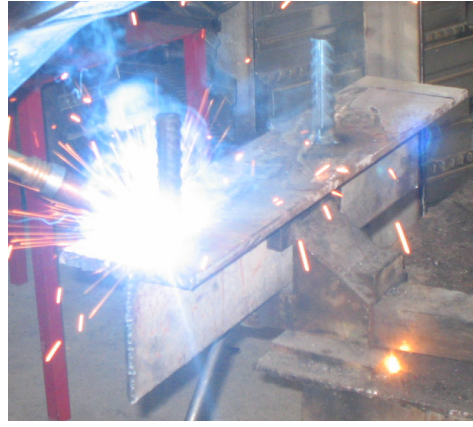
Figure 2. Earthquake resistant steel bar welded to the profile
