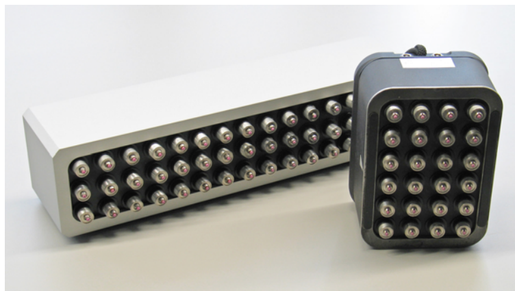
Fig. 4 Ultrasonic multi-channel array of 48 transducers in 16 groups (left), single-channel transducer of each 12 sending and receiving transducers, respectively (right)
