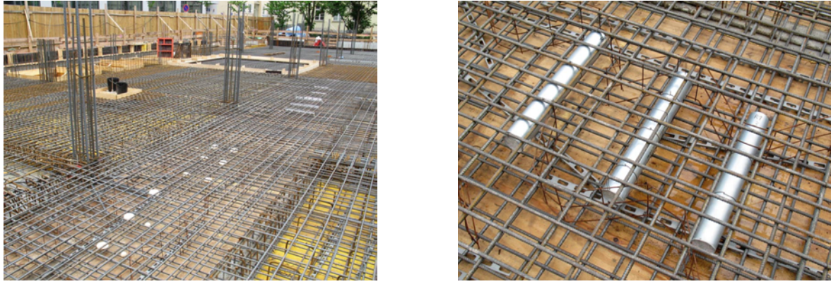
Fig. 6 Overview of the test site during construction (left); test field R1 with three pipes \varnothing 87 mm, divided in an empty part and a part filled with mortar
