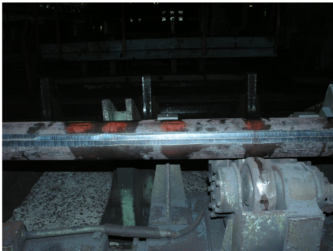
Fig. 7a. Bar with crack defect detected in course of testing at automated installation Volna-7
