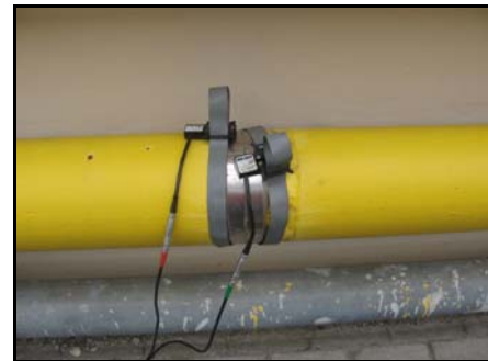
Fig. 1 - Magnetostrictive strip and coils applied on inspected pipeline.
