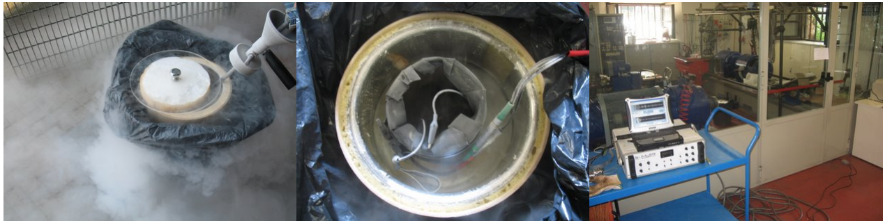
Fig. 5 – Test at -196^{\circ}\text{C} : (a) filling the Dewar; (b) piece of pipe and magnetostrictive guide wave sensor inside liquid nitrogen; (c) data acquisition.
