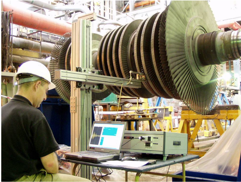
Fig. 8: Automated phased-array ultrasonic examination on blade attachment grooves in an HP/IP turbine shaft in Poland
