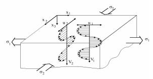
Combined equations (1,2) provide the evaluation of stresses in accordance with the nonlinear elastic properties of testing material and the results of precise time-of-flight measurements of shear and longitudinal ultrasonic waves:
