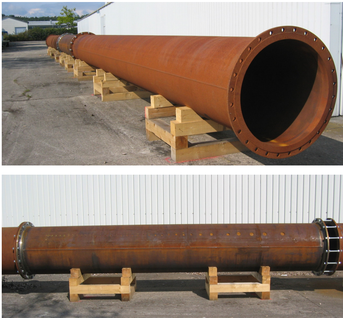
Figure 4.5: 40" test pipeline (top) containing test spool with artificial defects (bottom)
