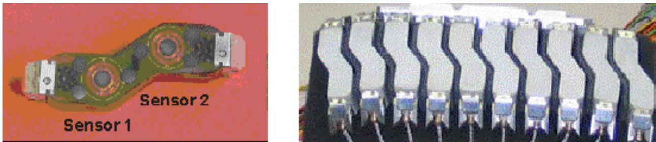
Figure 4.3: Left: basic unit containing two sensors (shown without wear plate). Right: unit with 20 basic units with ceramic wear protection. Each sensor measures ultrasonic (EMAT), MFL and EC signals.
