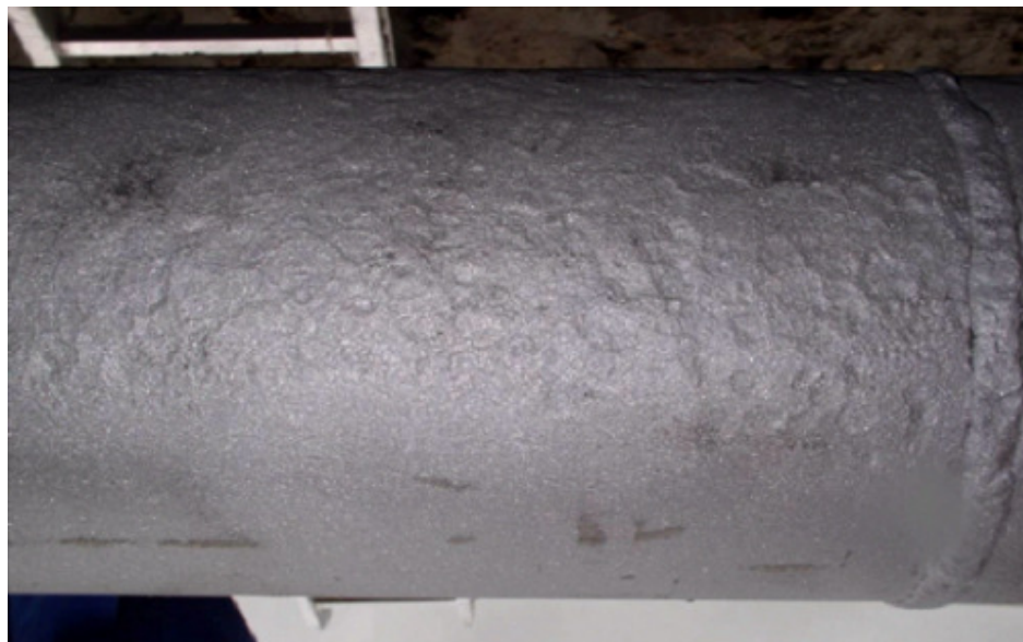
Figure 2.2: Example of external corrosion damage
