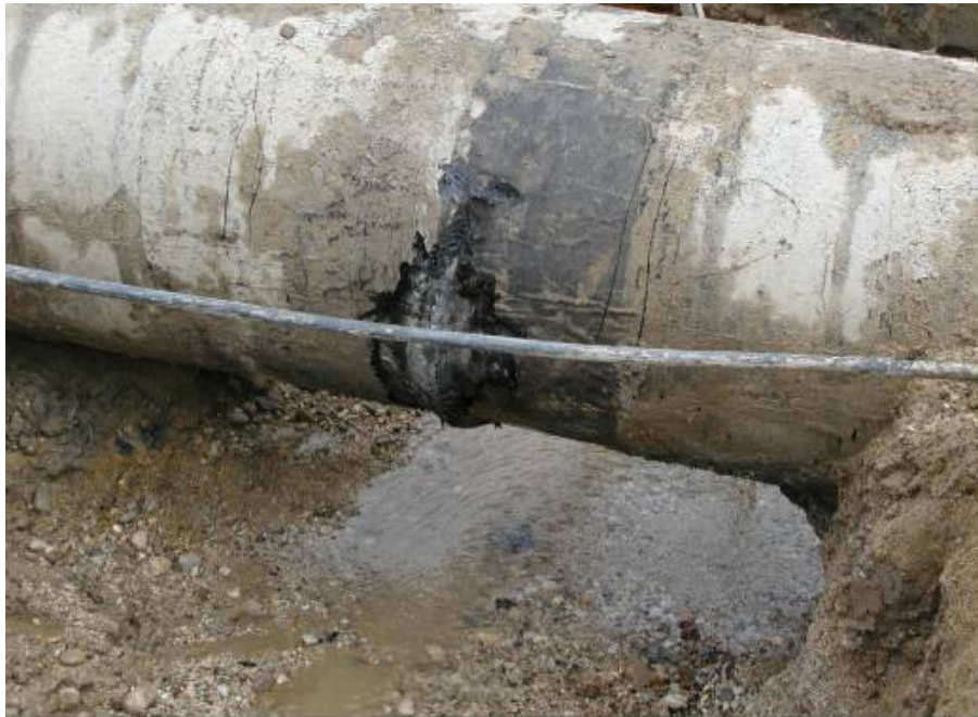
Figure 2.1: Example of deformation damage (wrinkle probably caused by landslide)
