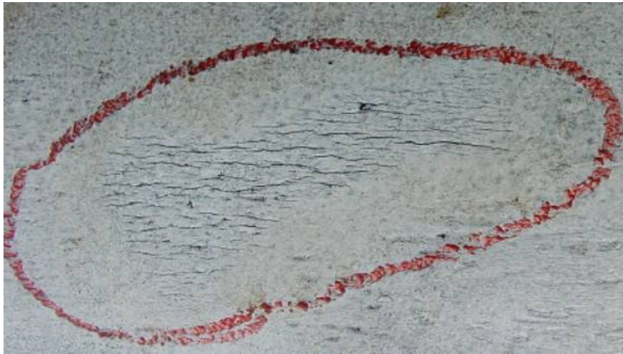
Figure 2.3: Example of an SCC colony
