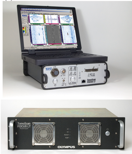
Figure 3: Top, Photo of Focus LT with laptop. Bottom, photo of Focus LT for PipeWIZARD V4
