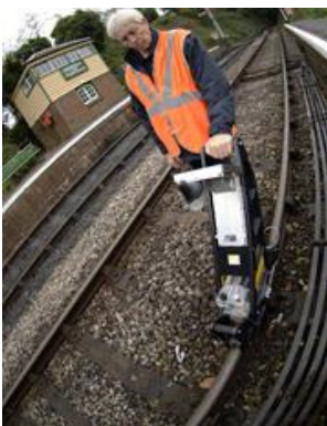
Figure 2: Sperry Rail's 'Walking Stick' non-contact magnetic rotary encoders contribute to rail track safety
