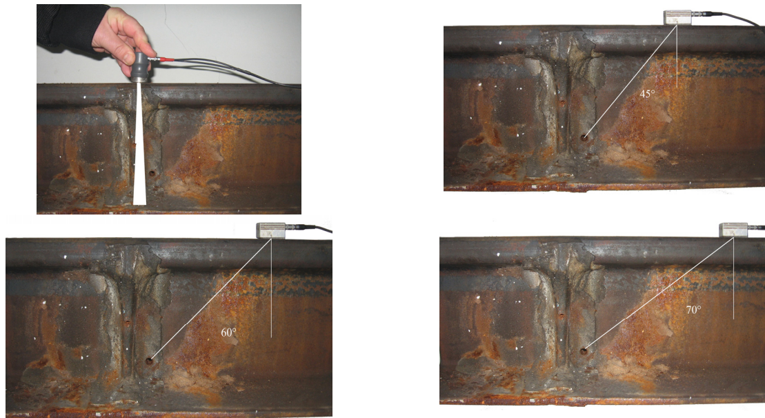
Fig. 3 Geometry of ultrasonic testing
