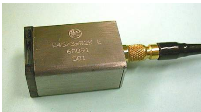
Pic. 14: MIC/MAC probe in sideview (left), and bottom-up
