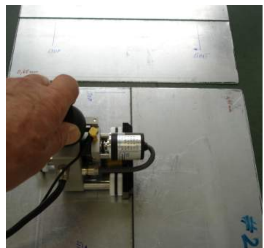
Pic. 20: Roller probe (WRL-B7), no motion encoding (left), with motion encoder (right)
