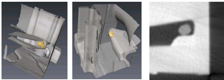
Figure 6 Sand core remain: segmentation (left, middle); CT image (right)
