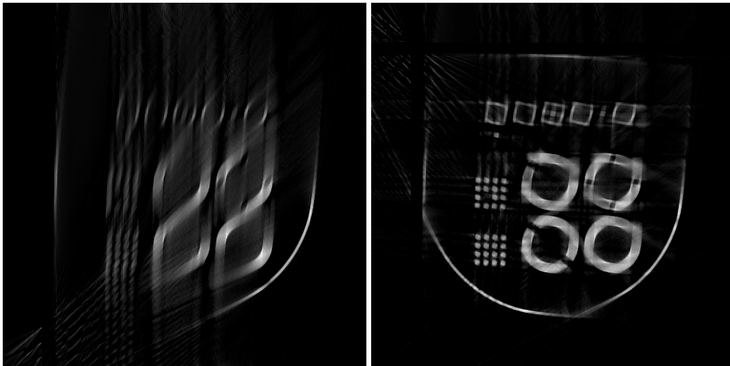
Figure 7: Reconstructions from translational data acquired during one translation (0°, left hand side) and during two translations in orthogonal directions (0° and 90°, right hand side)
