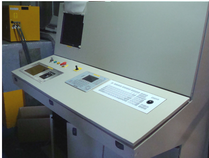
Figure 5: Control unit for the X-ray tube and the tomographic system.
