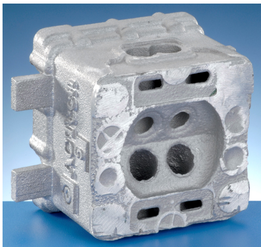
Fig. 1: The raw body of the new work-piece-near reference standard; state before segmentation and modification (block size 12 cm x 9 cm x 6 cm)
