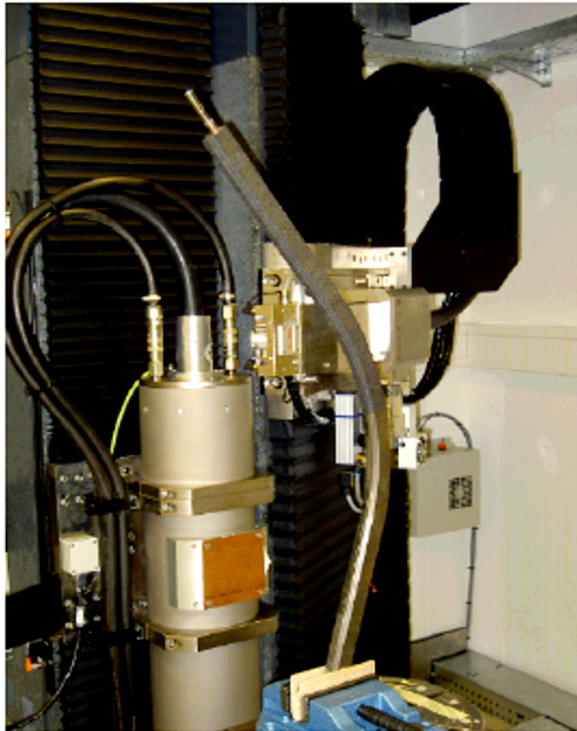
Fig. 7: Setup at the CT-device to scan vertical target of the ITER prototype (left picture). Cross-sectional CT-picture of the vertical target showing the CfC, the active metal casting layer and the CuCrZr (right picture).
