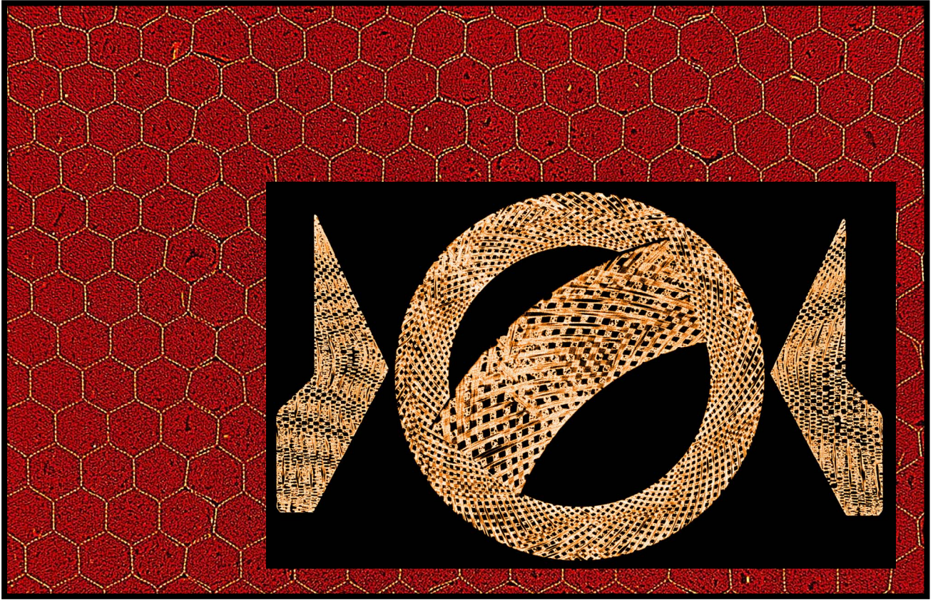
Fig. 6. CT images of honeycomb heat-protection block and carbon-carbon composite nozzle cluster
