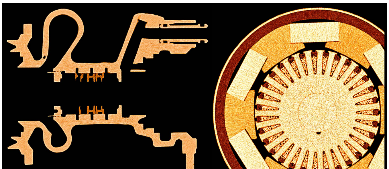
Fig. 5. CT images of steel airframe of liquid-fuel rocket engine and electric motor
