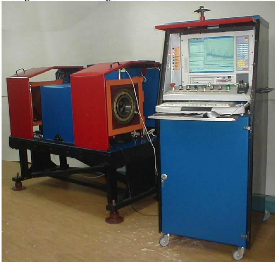
Fig.12. Stand for check in of rotor bearings for wheel pairs drive motor
