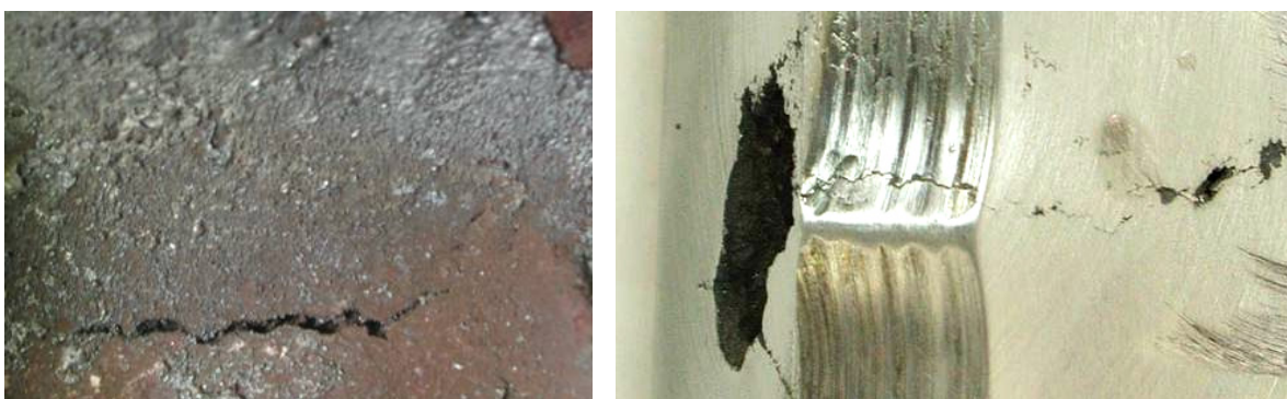
Fig.8. The defects detected in basic surface of bogie bolster using AE diagnostics
