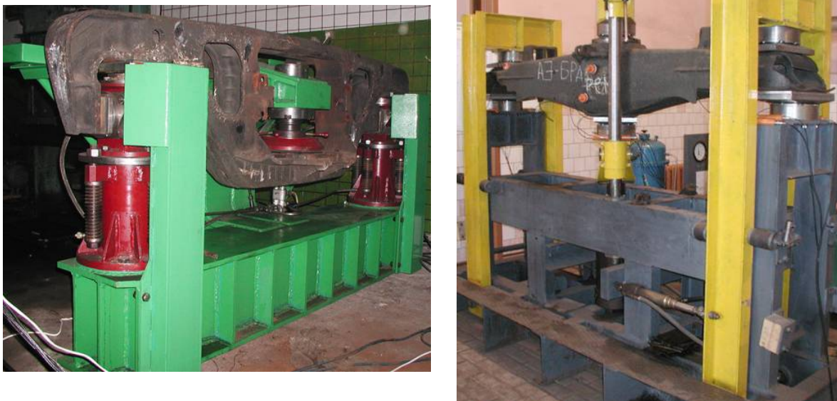
Fig.7. AE installation for freight-car truck cast details diagnostics (solebars and bogie bolster)
