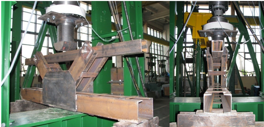
Figure 2: Full scale model of a steel bridge joint.
