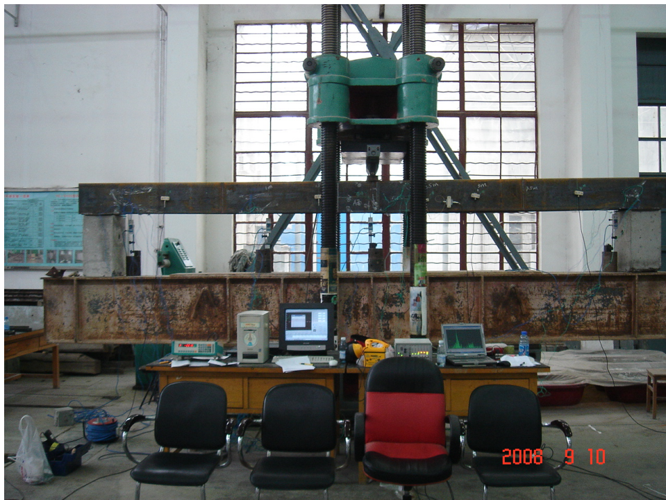
Fig. 2 Picture of AE testing for crossbeam
