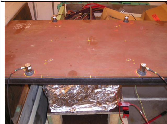
Picture 1: test set-up for corrosion tests under corrosive atmosphere without contact with liquid
