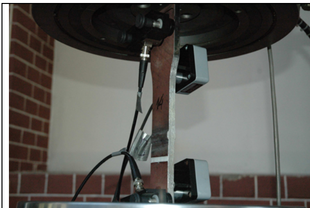
Picture 3: test set up for the fatigue on butt welded samples
