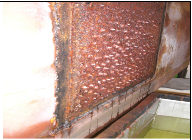
Picture 2: corroded test plate after first part of corrosion test
