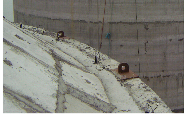
Figure 7: Intervention by a CETIM technician for the placement of sensors and their verification View of several waveguides ends;
