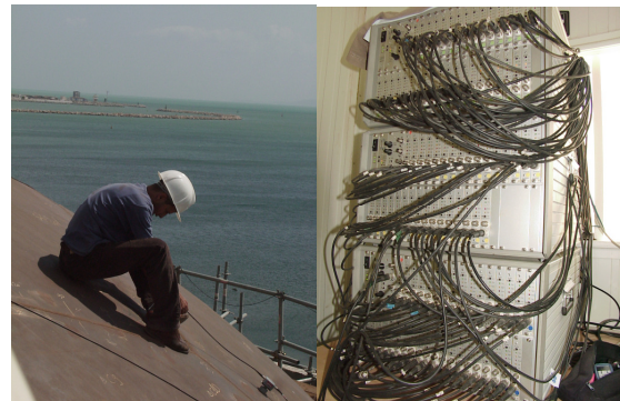
Figure 4: Installation and sensitivity checking of the sensors by a qualified operator – AE System VALLEN AMSY-5 104 channels
