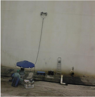
Figure 3. Industrial Automated Ultrasonic Crawler (LSI) during scanning of tank wall
