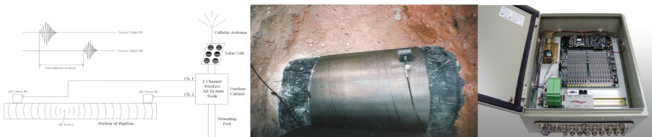
Figure 12. AE Remote Pipeline Monitoring system.
