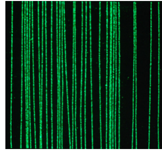
Picture 2: Cracks indication on Ni-Cr Panels, after treatment with MET-L-CHEK aerosol penetrant system. Dwell time 10 min, development time 3 min., room temperature, defects width 0,25 \mu\text{m} , defects depth 5 \mu\text{m} – left photo, defects width 0,5 \mu\text{m} , defects depth 10 \mu\text{m} – right photo.
