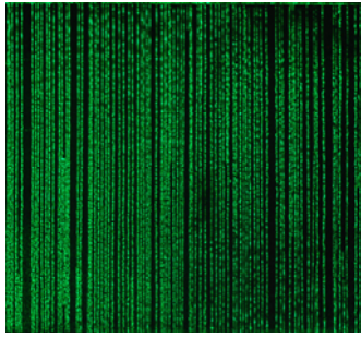
Picture 2: Cracks indication on Ni-Cr Panels, after treatment with MET-L-CHEK aerosol penetrant system. Dwell time 10 min, development time 3 min., room temperature, defects width 0,25 \mu\text{m} , defects depth 5 \mu\text{m} – left photo, defects width 0,5 \mu\text{m} , defects depth 10 \mu\text{m} – right photo.
