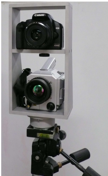
Figure 2: Frame for a stable connection between visual and IR camera.
