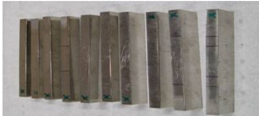
Figure 4: mock-ups with calibrated depth cracks and the associated calibration curves
