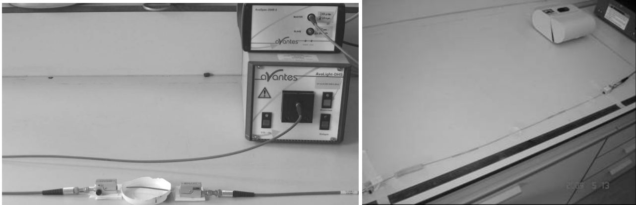
Figure 3 left) The sensing part of the optical fibre sensor is protected by a perforated tube, right) “long fibre” sensor set-up with different sensing spots
