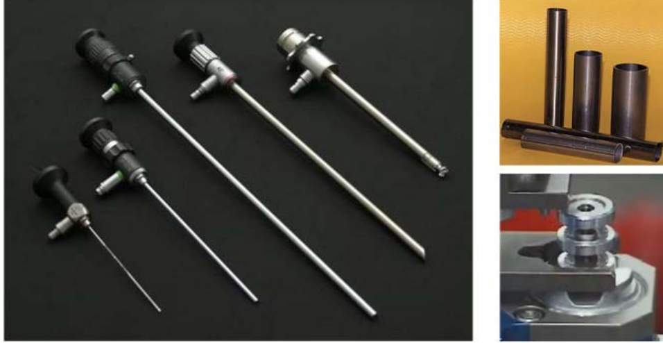
FIGURE 1. Standard endoscopes (also called borescopes) with different diameters and typical industrial inner surface examples.
