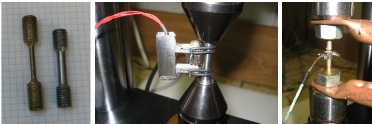
Fig. 8. From left to right: a) typical samples; b) investigated steel sample with mechanical extensometer; c) sample heating by direct current.
