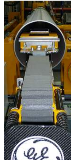
Figure 8: Pipe inspection with DXR 250RT-E
