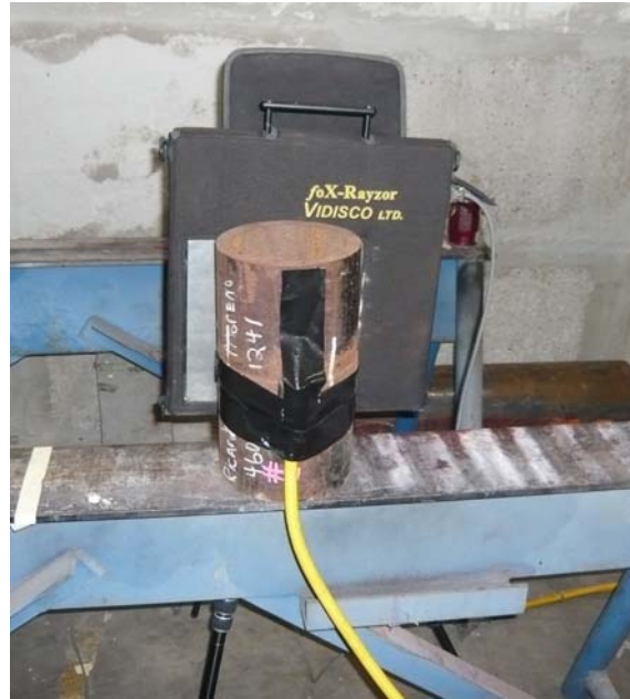
Figure 6: External Setup; foX-Rayzor mounted on Tripod and Radioactive Source (Contact Method)
