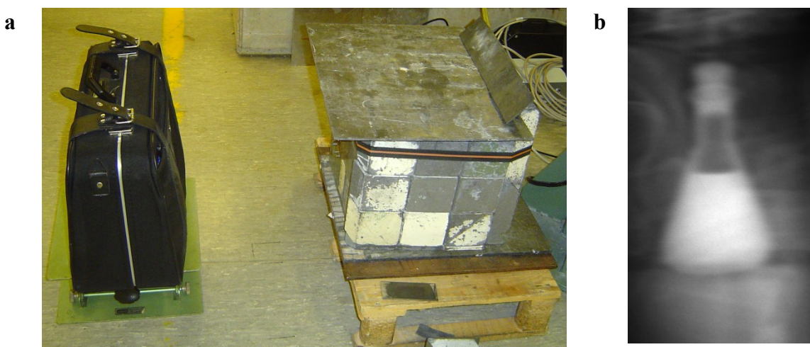
Figure 4: Erlenmeyer flask filled with water and sealed with a rubber bung hidden in a packed suitcase, a) experimental setup, b) backscatter image of the hidden object encased by odds and ends.
