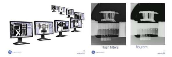
Software is a key element for all digital solutions and brings the differentiation with film. More tools are available which enable the user to communicate faster and to enhance images using window leveling and wall thickness measurement is automated and more accurate. Complex mathematical analysis methods can be used with little effort for the end user.
