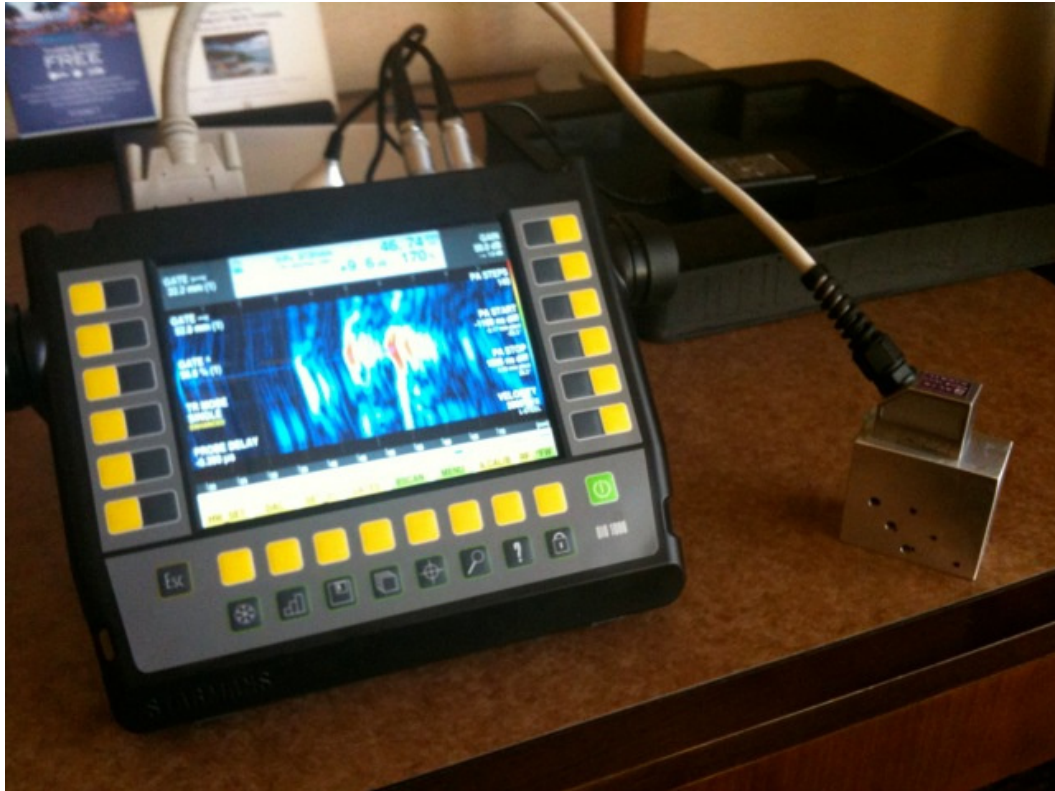
Fig. 6. Material scanning using phased array technology
