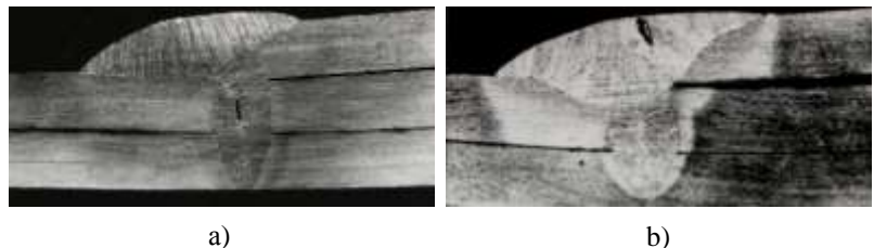
Fig. 11. Flaws in multi-layer shell weld seam detected by EMA equipment: a) lack of fusion, b) pore
