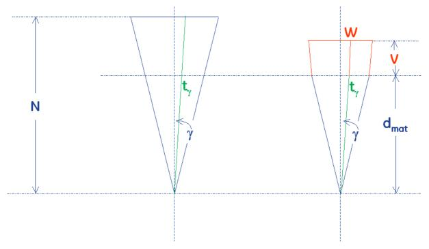
On the left side the straight beam probe without delay line is illustrated. On the right side is the constructed straight beam probe with the given delay line length of v.
