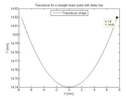
The slight paraboloid shape results in a defocusing effect. The following figures compare the probe used for construction (red) and the resulting probe with the paraboloid transducer (blue, left figure) and a probe having a flat transducer with the same size (width) as the paroboloid transducer (right figure). The longer near field length to be seen in the left figure shows the defocusing effect.
