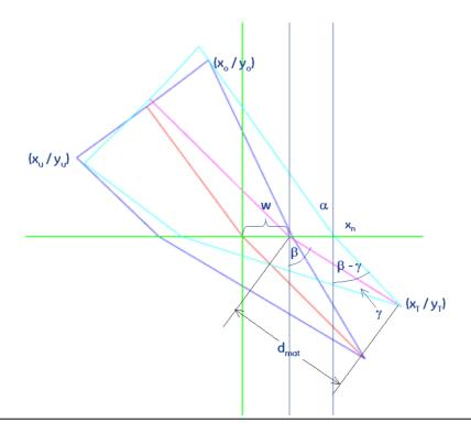
The task to perform is, to calculate  $d_{mat}$  and the shift of the sound index point w in a way that the edge sound beams of the virtual transducer are going through the corresponding edges of the original transducer.
