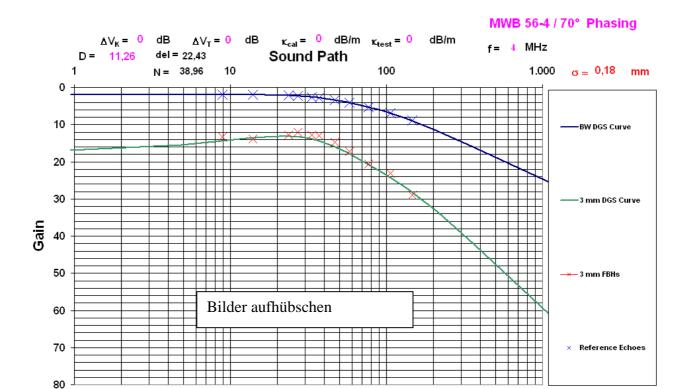
Though following the presented model the transducer shape would be different from the used transducer for the three different angles, one can directly see from the results that also for phased array probes the agreement of expected and measured gain values at given distances is noticeably accurate and lies in the same range as for the single element angle beam probe shown above.
