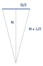
At the end of the near field the difference between the central beam and an edge beam defining the outer perimeter of the transducer is  $\lambda/2$  (or equivalent, the time of flight difference between central and edge beam is T/2), with  $\lambda$  = wave length in the material, T = 1/f and f = probe frequency.
