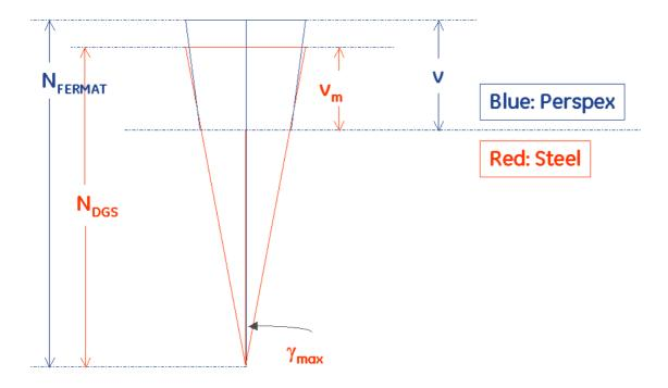
To calculate the near field length of a circular transducer completely in steel (trans) the angle  $\gamma_{max}$  is used and the fact that the difference between the central beam and one edge beam needs to be  $\lambda/2$ :
