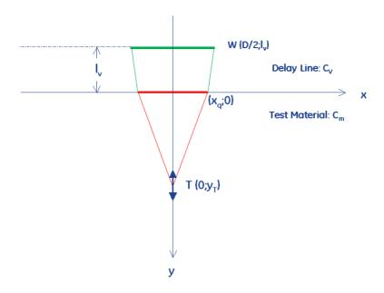
Here the time of flight t from point W to point T is calculated in dependency of y<sub>T</sub>:
