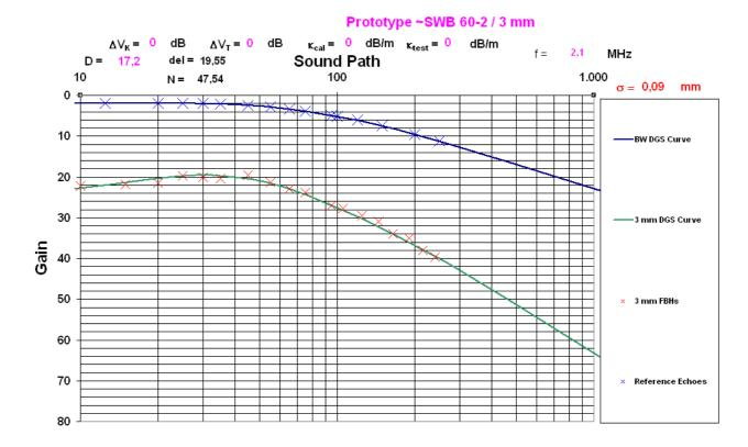
This new probe shows a noticeable good agreement with the DGS-diagram over the complete measurement range. The deviation from the expected gain values at a given depth decreased to a standard deviation  $\sigma$  of only 0.09 mm, taking all measured values into account.
