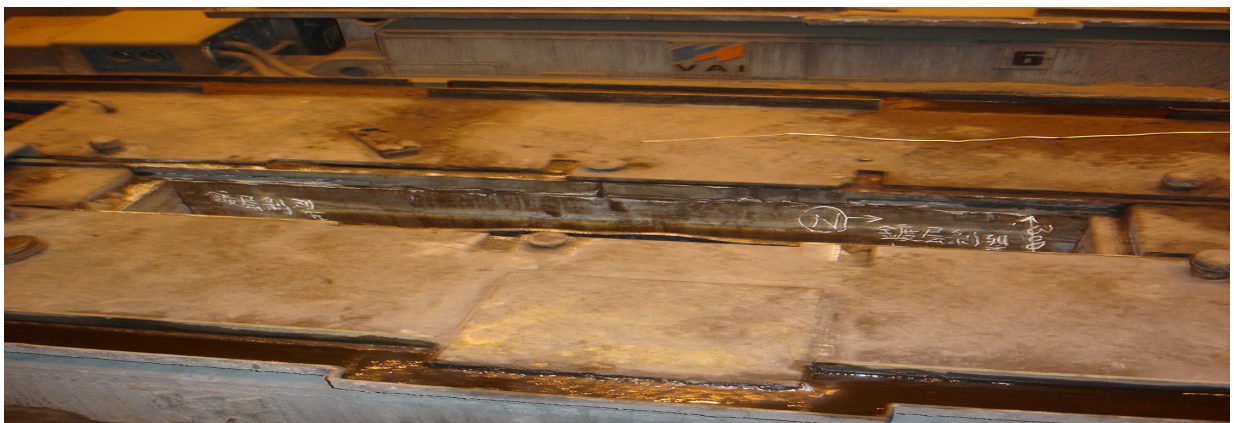
Figure 2. Short distance top view of Mold of casting machine in pouring gate
