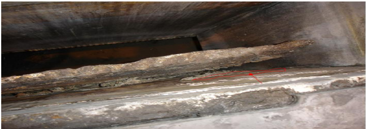
Figure 4. The nickel layer split off from the copper mold
