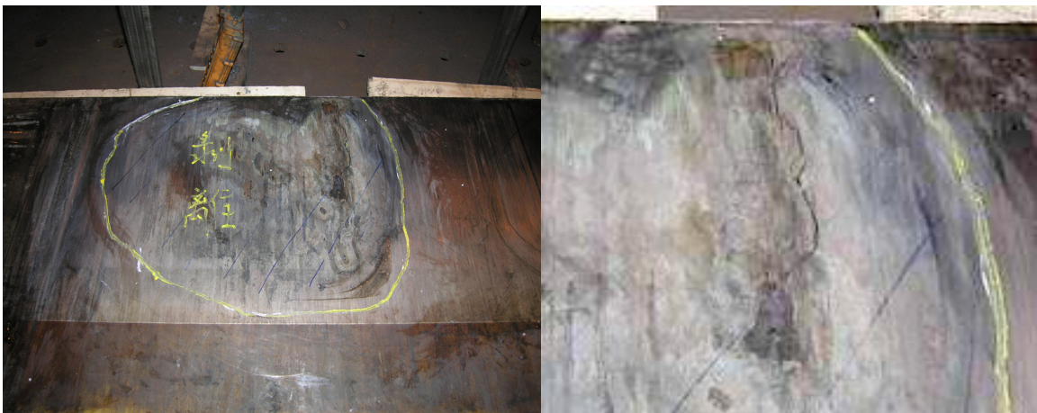
Figure 5. Left is the surface fissure of copper mold and right figure is close shown
