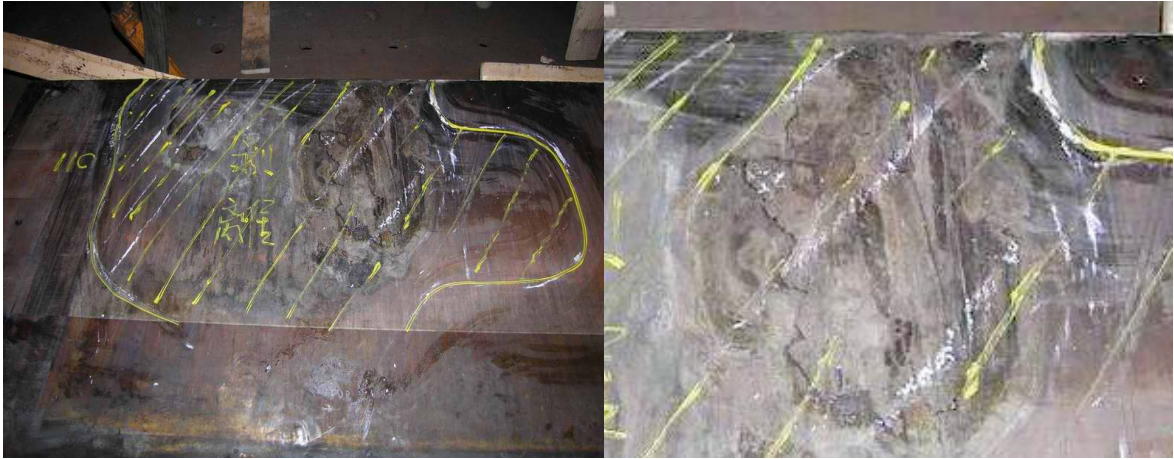
Figure 6. Left is Split off area of nickel layer of copper mold and right figure is close shown
